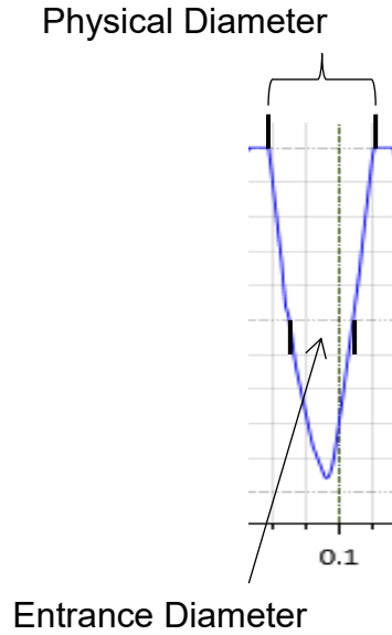
Fig. 32: Potential profile of a grid. The entrance diameter is where the valley crosses a value of 500 V while the physical diameter is the physical diameter of the grid hole.
