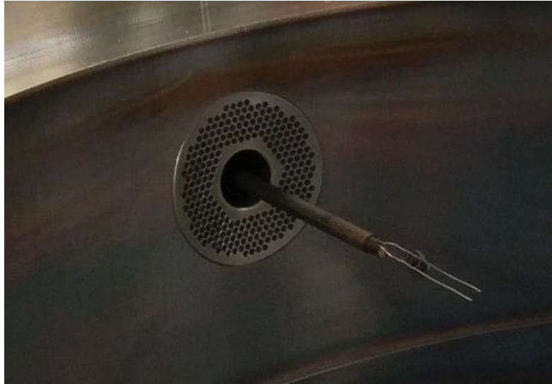
Fig. 134: Picture of the hairpin resonator probe (or hairpin) and corresponding port cover in the chamber wall. The port cover was designed to allow the hairpin to move in and out while trying to prevent light-up in the hairpin housing connected to the chamber wall
